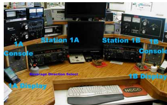
SO2R Station 1 showing the antenna select operator interface.
