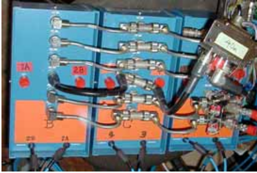
Figure 4. The Antenna-Band Matrix consists of three “SixPaks”
