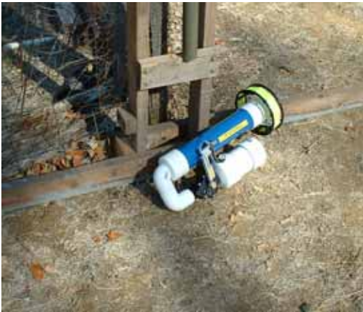
K6SRZ's (W6PZ) secret weapon for CQP: the WB6ZQZ tennis ball launcher. This will put an antenna line 150 feet in the air!
