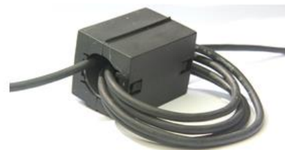
Fig 7 - 5 turn choke, good for 7-30 MHz
