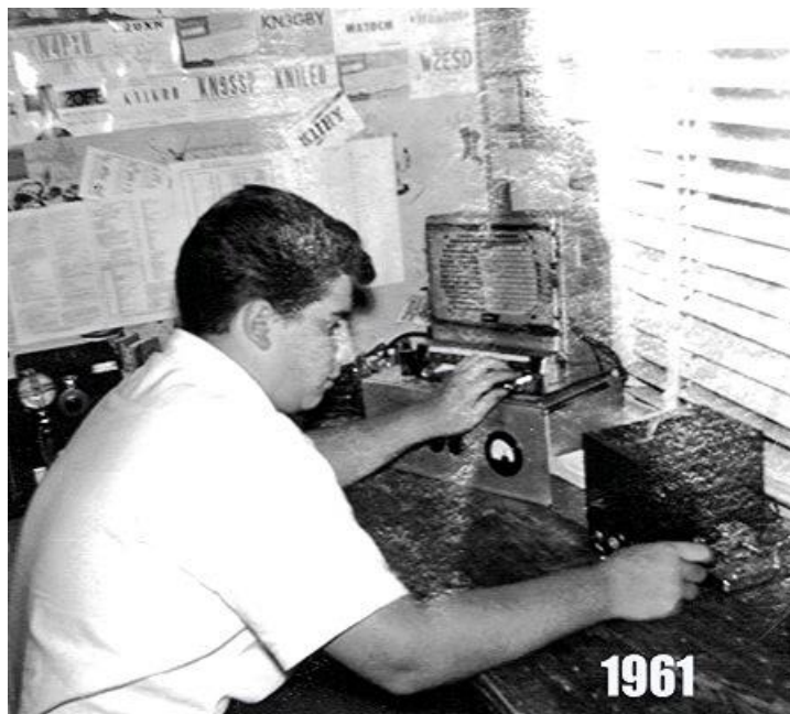
WA2GGB 1961 – Talk about a primitive station. Operating 6M CW. 5W transmitter. 6M Nuvistor converter into a car radio. Signal generator at 455KHz for a BFO. 3 element Cush Craft beam at 8 feet.
