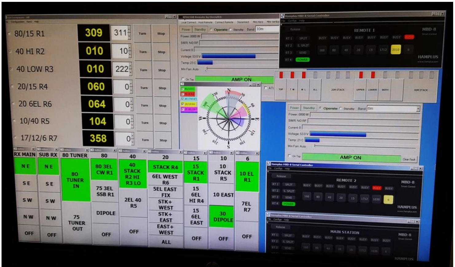
CONTROL SCREEN – All antenna switching, rotor control, phase box control, remote amps and remote switch monitoring on one touch screen. Remote operators’ access this through TeamViewer. W1YL is the star of the remote operators with 2,349 QSO’s in 2018.
