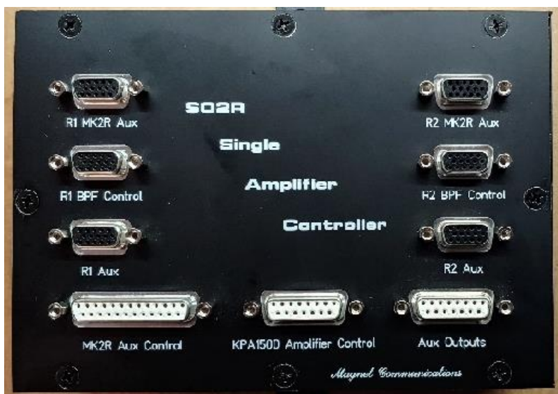
Figure 3. Controller Panel for K6MR’s KPA-1500 SO2 Configuration.
