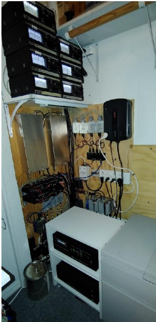
Figure 5. The KPA-1500 K6MR SO2 System Installed in a closet near the K6MR Shack
